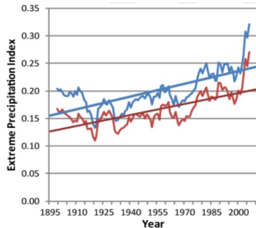
Figure 3: Time Series of extreme precipitation index for the occurrence of 1-day, 1-in-5-year extreme precipitation events. The annual time series and linear trend (straight line) are shown in blue. A time series for the months of May through September is shown in red. Analysis is average for the states of IL, IN, IA, MI, MN, MO, OH, and WI. Based on data evaluated in (Kunkel et al., 2013).
