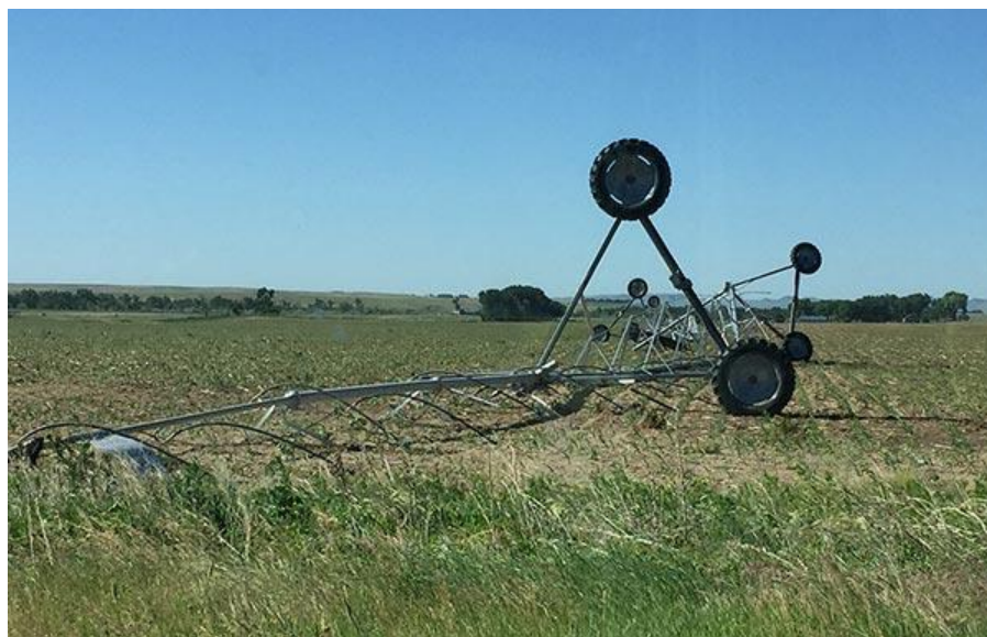
Center pivot flipped by strong winds. Photo courtesy of National Weather Service, 2017
