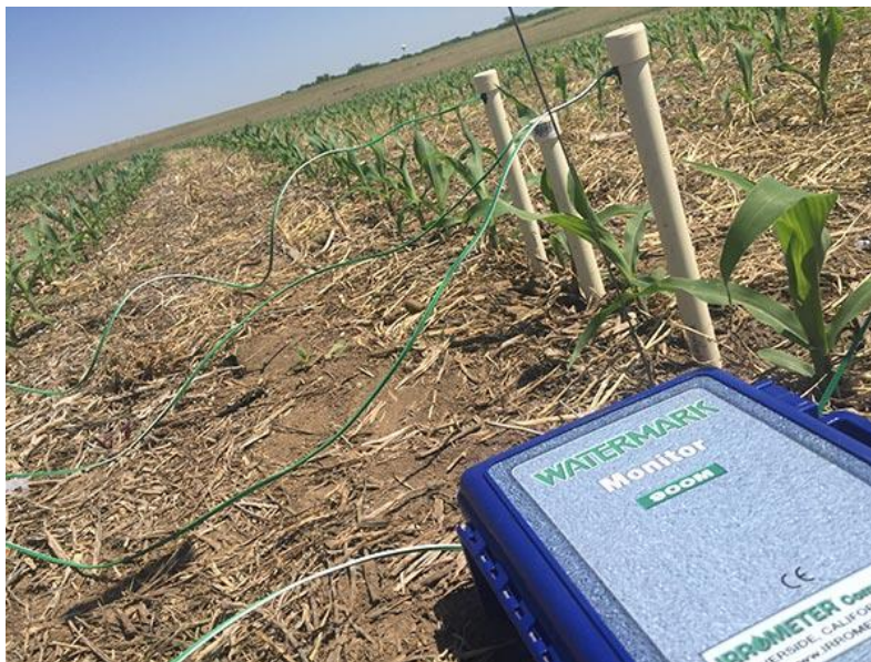
Soil moisture sensors are a great way to increase irrigation efficiency. Photo from Tyler Williams, University of Nebraska, 2018.
